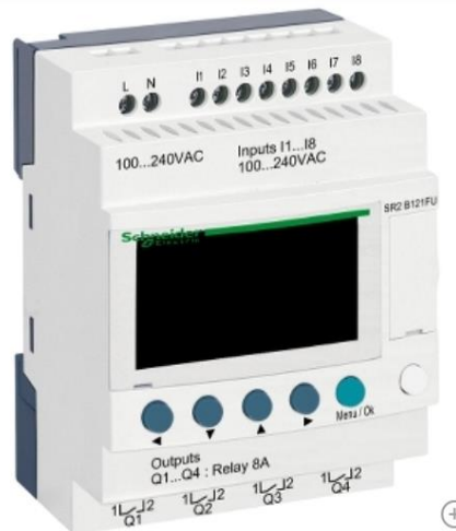
Fig.4. The SR2 B121FU Zelio PLC
